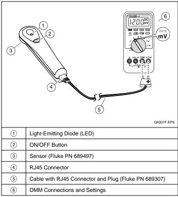
Fluke CO-210 Carbon Monoxide Probe
